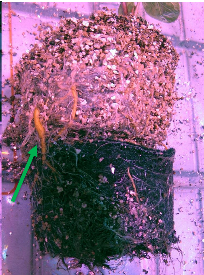
Figure 9: Sample removed intact from pot. In this control sample, roots bind the vermiculite and compost layers into separate solid 'root balls', and bind the fabric disc to both the vermiculite and compost layers. Despite precautions, some roots have grown around the edge of the fabric disc (green arrow).
