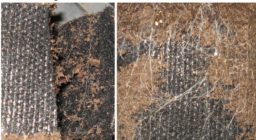
Figure 5: In soil, roots of Arabidopsis thaliana can grow in close proximity to CuTex without obvious inhibition.
